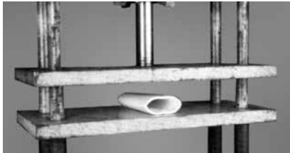
PVC Conduit PVC conduit will stay compressed if it is crushed. (Same for steel conduit.)
