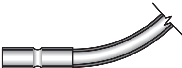
Deep Socket PVC Coupling bonded onto fiberglass elbow
