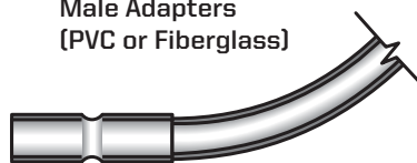
Deep Socket PVC Coupling bonded onto fiberglass riser
