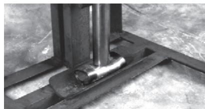
For high-impact, steel conduit will collapse and can pinch the cable. This will make repair of damaged conduit more difficult.
