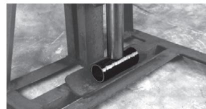
XW conduit has the highest impact value of all conduit materials available. If impacted, it will flex back close to its original diameter. SW, MW and HW will also flex back similarly after impact. They will not shatter.
