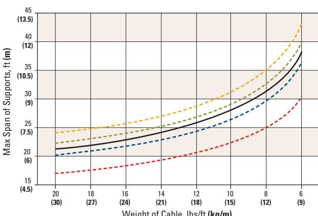
It is recommended that mid-span deflection never exceeds 5/8 in (16 mm).
