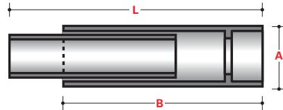
**SINGLE EXPANSION JOINT SOCKET X SPIGOT WITH O-RING**
