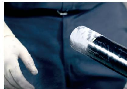
Apply the Champion Mix® two-part epoxy adhesive to the conduit ends. NEVER apply adhesive to the inside of sleeve couplings or fitting sleeves as this could potentially cause the adhesive to drip inside the conduit/ fittings and possibly interfere with the cable pulling process. Champion Mix is designed to permanently bond fittings and the joints of fiberglass reinforced epoxy conduit. It is also designed for use with pultruded polyester and vinyl ester fiberglass components.
