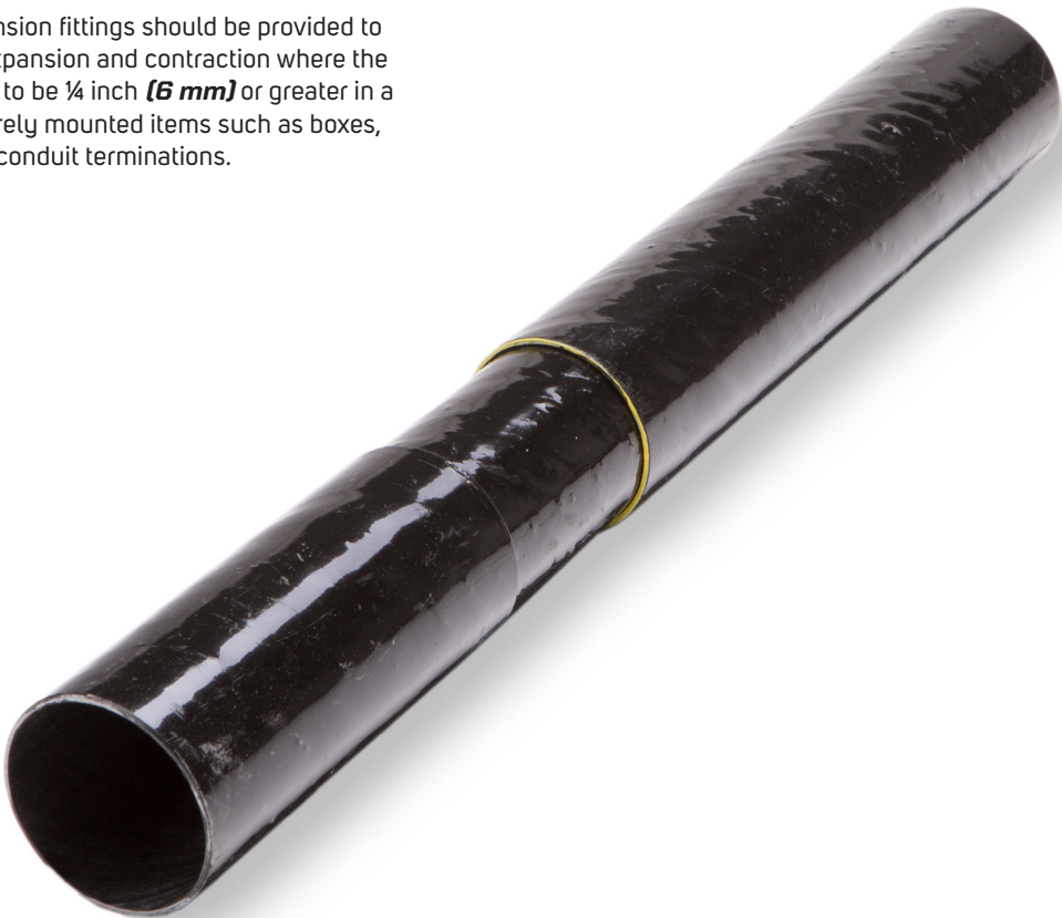
Expansion Characteristics of Champion Fiberglass Reinforced Thermosetting Resin Conduit (RTRC) Coefficient of Thermal Expansion = 1.2 x 10-5 in/in/°F (2.2 x 10-5 m/m/°C)
