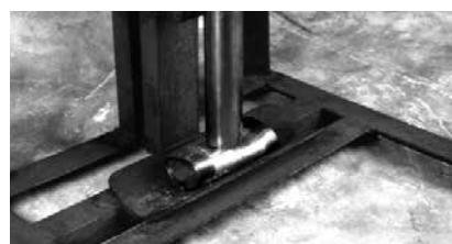
For high-impact, steel conduit will collapse and can pinch the cable. This will make repair of damaged conduit more difficult.
