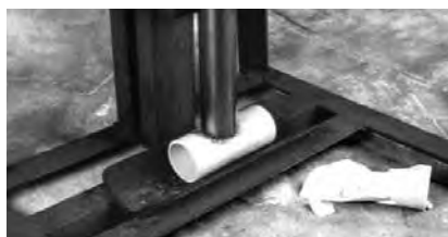
For high-impact situations as well as during cold weather, PVC can shatter and/or flatten.
