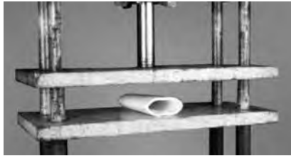
PVC Conduit PVC conduit will stay compressed if it is crushed. (Same for steel conduit.)
