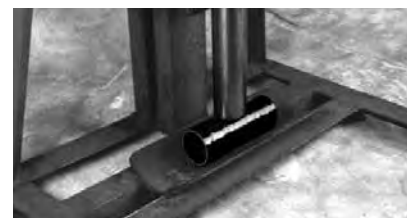
XW conduit has the highest impact value of all conduit materials available. If impacted, it will flex back close to its original diameter. SW, MW and HW will also flex back similarly after impact. They will not shatter.
