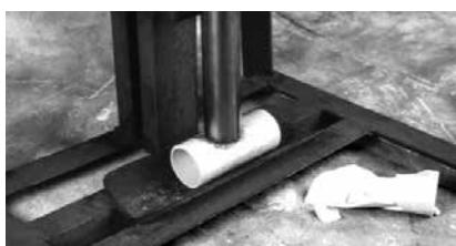
For high-impact situations as well as during cold weather, PVC can shatter and/or flatten.
