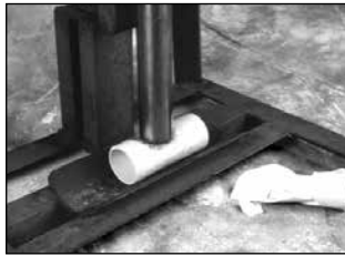
For high impact situations as well as during cold weather, PVC can shatter and/or flatten.
